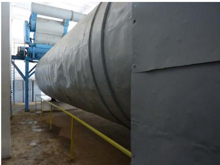
In the gin the seed cotton is dried in very large rotating drums, though which air is passed, the temperature depending on the measured humidity, rather like a clothes drier, but on a larger scale. A system that the Committee applauds as a manner to gently dry without damaging the cotton fiber. After this process the cotton travels first to a horizontal cleaner, unique for the central Asian countries, and then on to a vertical pre-
